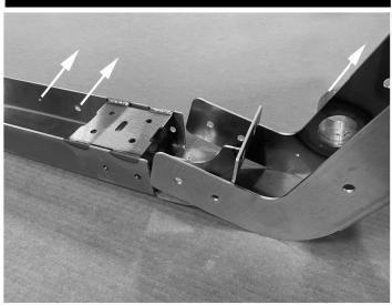
1. Install each leg to the transverse cross member. Use (6) 3/8"x1.00" button head bolts and flange lock nuts for each corner. Do not tighten securely. Make sure holes on the transverse cross member and gate pivot tube are facing the same direction.
