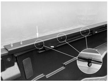
12. Install the driver side base rail as shown above. Run the LED harness along the inside of the base rail. Use the supplied push rivets and wire clamps. There should be approximately 70 inches of the end of the harness extending beyond the hole marked with an arrow.
