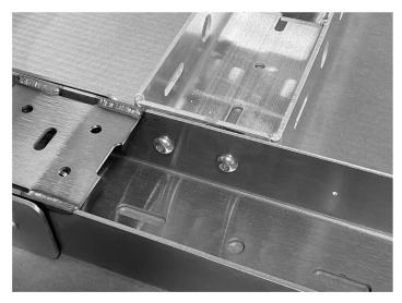
5. Connect the opposite side longitudinal cross bars as shown. Use (2) 3/8"x1.00" button head bolts and flange lock nuts. Torque to 30 ft/lb.
