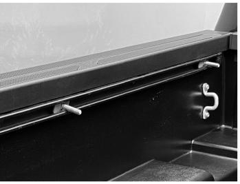
11. Install (6) track inserts as shown to both sides of bed. Use the base rails from step #9 as a guide for location.
