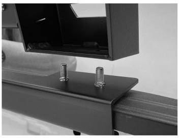
15. Install the assembled rack to the base rails on one side of the vehicle.
