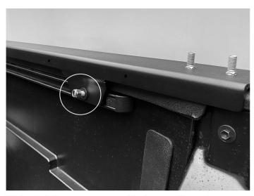
13. Install the passenger side base rail as shown above
