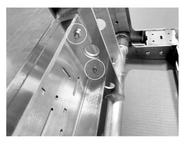
7. Close the gate door and lock into legs using (4) supplied pins. Install the accessory mount panel as shown using (4) 1/4" x 3/4" hex bolts, washer and nuts.
