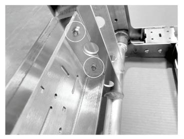
8. Close the gate door and lock into legs using (4) supplied pins. Install the accessory mount panel as shown using (4) 1/4 x 3/4 hex bolts, washer and nuts.
