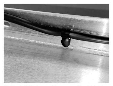
10. Route LED wires and harness on the right side of the vehicle using supplied wire clamp and push rivits as shown on the inside of the bed rails and cross bar assembly. Each leg and transverse cross bar has (9) holes, Each base rail has (7) holes.
