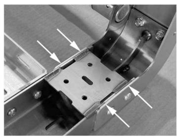
2. Align the leg with the transverse cross bar and tighten all fasteners. Torque to 30 ft/lb. Confirm leg flanges are parallel with cross bar as shown.
