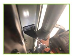
2) Locate the (2) bolts for each of the (4) mounting points found on the underside of the truck. Using a metric socket and power drill remove each side step.
