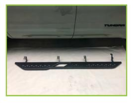
3) Prepare the ZROADZ Side Step for install. Identify the Driver / Passenger Side Step by having the ZROADZ logo right side up as you mount it. Use the help of another person to mount the side step.
