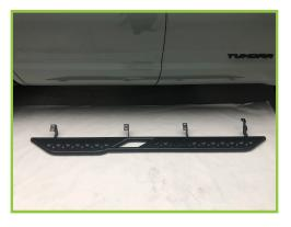
3) Prepare the ZROADZ Side Step for install. Identify the Driver / Passenger Side Step by having the ZROADZ logo right side up as you mount it. Use the help of another person to mount the side step. **STEP 4**
