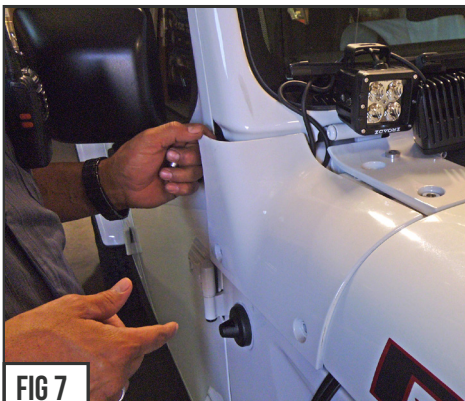
STEP 6 INSTALLERS NOTE: Mock Up LED Lights and plumb wires.
