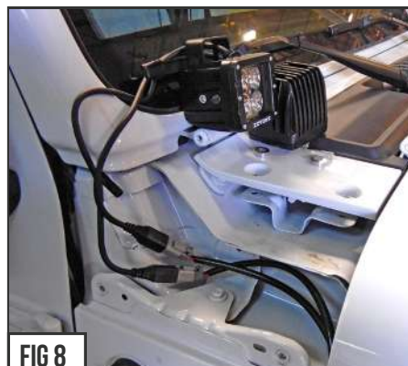
STEP 6 INSTALLERS NOTE: Mock Up LED Lights and plumb wires.
