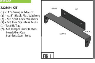
1) Begin by taking the ZROADZ Brackets and note where the ZROADZ Bracket mounting slots are located and that they will mount on the backside of front bumper.
