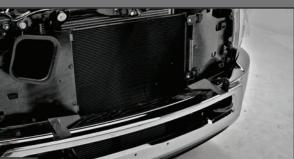
STEP 1 1) With the hood open and bumper accessible, mock up and put into place the supplied bumper LED Mounts. This will help you gain familiarity of how and where the brackets will mount onto the vehicles front bumper.
