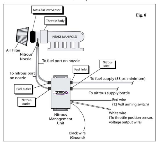
B. Take the black wire that comes from the Nitrous Management Unit and attach it to a suitable chassis ground. Remember to remove any paint at the attachment point to ensure a good ground.
