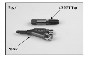
the spray is in the direction of airflow. We've also enclosed a tap (Fig. 6) should you desire to mount the nozzle directly into a metal air intake tube. Just drill an 11/32 inch hole where you want to thread-in the nozzle, tap the hole and install the nozzle. Once installed, place the appropriate tuning jets in the nozzle and attach the 2-foot long, -3AN hoses to the nozzle jet fittings and the Nitrous Management Unit (Fig.5).
