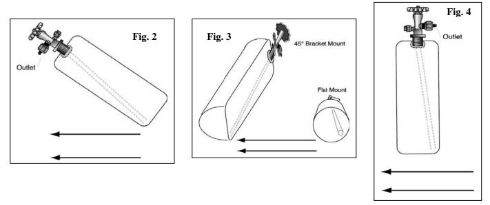
2. Mount nitrous supply bottle - Mount the nitrous supply bottle so that it is separated from the passenger cabin. Fastback style cars that do not have a separate trunk compartments have to be equipped with a safety blowdown tube (Fig. 5). Route the tube from the safety pressure relief
