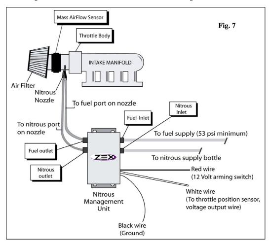
D. Take the black wire that comes from the Nitrous Management Unit and attach it to a suitable chassis ground. Remember to remove any paint at the attachment point to ensure a good ground.
