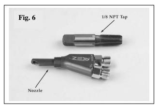
your engine. Install the nitrous nozzle so that the spray is in the direction of airflow. We've enclosed a tap (Fig. 6) should you need to mount the nozzle in a metal duct. Just drill a 11/32 inch hole where you want to mount the nozzle, tap the hole and install the nozzle. Once the nozzle is installed, place the appropriate tuning jets in the nozzle and attach the 3-foot long, -3AN hoses to the nozzle jet fittings and the nitrous management unit (Fig.5).
