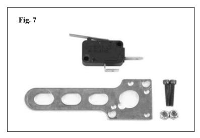
**C.** The throttle switch bracket is made of easily formed material. Attach the end of the bracket to one of the throttle body studs and bend the bracket in such a way to allow the throttle arm to contact and depress the switch's lever at wide open throttle.
