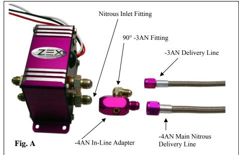
3. Attach and tighten the -4AN in-line adaptor to the NMU/nitrous solenoid inlet fitting. At this point, you may turn the inlet fitting with the in-line adapter tightened to it, clockwise, to achieve the desired inline adaptor position. The inlet fitting uses a pipe thread, so the additional turning in the clockwise direction should be kept to a minimum. Do not overtighten the inlet fitting (Fig. B).
