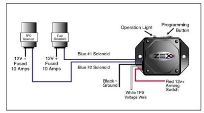
armed and ready to activate at wide-open throttle. Return to the driver's seat and depress and release the accelerator pedal several times. You should hear the solenoid click each time you reach wide-open throttle. At this point, your ZEX<sup>TM</sup> Programmable TPS switch is fully programmed and ready for use. If you ever transfer your nitrous system to another vehicle, perform this same procedure on the new vehicle to "relearn" the TPS switch.
