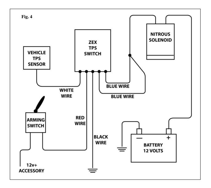
7. **Program TPS Switch.** To program the switch, turn the vehicle's ignition on, but do not start the engine. Turn the nitrous arming switch to the "ON" position. Go to the ZEX<sup>TM</sup> TPS switch and locate the programming button on the top of the housing. Depress, then release, the pushbutton switch. Observe the unit's Operation Light. At this point, it should be RED. This RED
