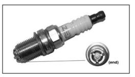
nitrous accelerated burn. The correct solution is to replace the plugs with units that have shorter ground straps. By doing this, you will shorten the heat path from the ground strap to the plug base. ZEX<sup>TM</sup> Hyperformance<sup>TM</sup> spark plugs are recommended for many applications.
