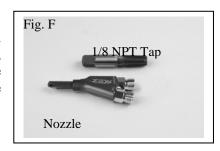
duct from your engine. Drill a 9/16-inch mounting hole and install the bulk head fitting. Be sure to remove any drill shavings since they can severely damage your engine. Install the nitrous nozzle so that the spray is in the direction of airflow.
