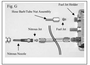
Nitrous Management Unit gets connected to the vacuum fitting on the engine's fuel pressure regulator with one of the lengths of hose. The intake hose barb from the Nitrous Management Unit gets connected to an unused vacuum fitting coming off of the intake manifold plenum with the other length of hose. Install the fuel tuning jet in the holder as seen in Fig. G and tighten the hose barb / tube nut assembly over the top of the jet.
