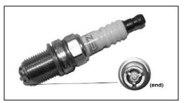
solution is to replace the plugs with units that have shorter ground straps. By doing this, you will shorten the heat path from the ground strap to the plug base. ZEX<sup>TM</sup> Hyperformance<sup>TM</sup> spark plugs are recommended for many applications.
