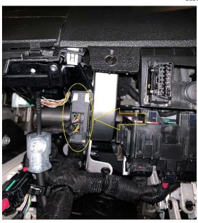
Installation is a matter of unplugging the SGW module above the OBD2 diagnostic connector and plugging the Tazer DT in its place. Simply locate the SGW and unplug its two connectors by pressing the tab with
