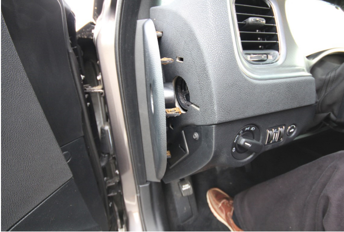
Removal of side panel; pulls off.
