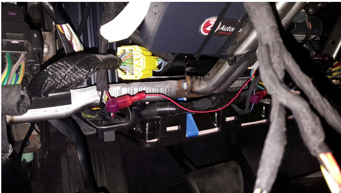
Power wire tapped and connected to OBD2 harness.
