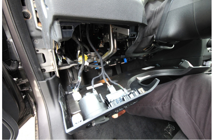
Remove 2 screws; pull lower cover straight back.
