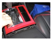
**Step 3:** Remove the cover in front of the ashtray. This simply pulls up. Underneath are two Philips head screws to remove.
