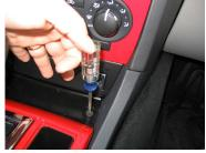
**Step 4:** Disconnect the wire to the radio bezel and set the bezel aside. Pull the ash tray out. Remove the wiring to the cigar lighter, and seat heat switches, if equipped.
