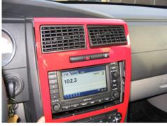
**Step 2:** Pull out the shifter tray. Insert finger in hole on side of bezel(in the tray area) and pull up on bezel to pop the snaps. Do not pull up on the front of the bezel, as it is still held in place by two screws near the ash tray.
