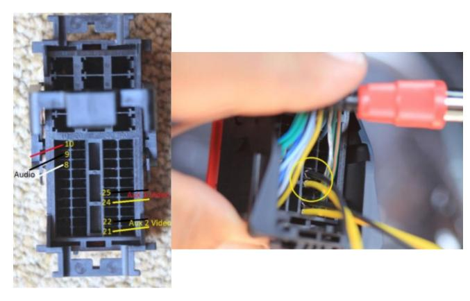
Once the cover is raised, insert the pins of the supplied RCA cable into their proper slots.
