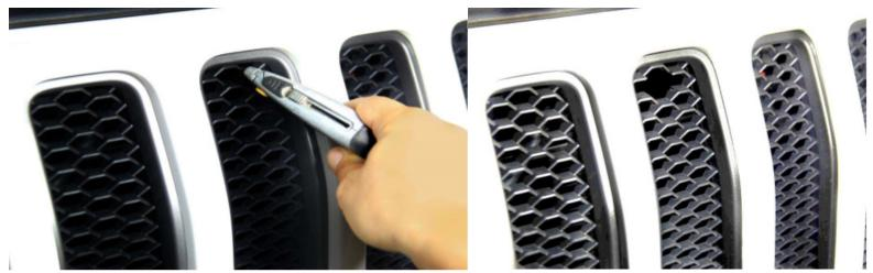
Using a box cutter or wire snips, trim middle grill slating to fit camera bracket.
