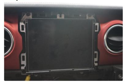
Using a phillips head screwdriver remove the 4 screws holding the radio into the dash.
