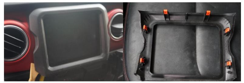
Once screws are removed, use a trim stick to remove bezel from dash.
