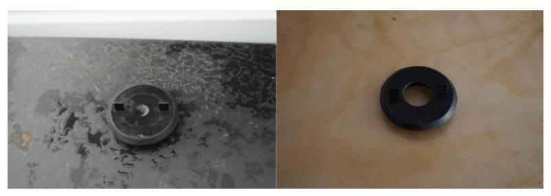
Remove clutch plug located on the firewall below the brake booster on the driver side. Using a 1/2" drill bit, drill a hole in the center of the plug to route the wiring into the vehicle. It is recommended to use a grommet or silicone to seal the wiring in the plug.
