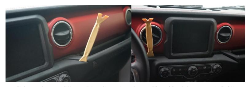
Using a trim pry stick, carefully release the tabs on either side of the center dash AC Controls. Once Released, unplug the two connectors on the back.
