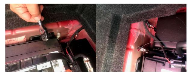
Plug in your Z Automotive device or other compatible OBD2 device and enjoy. A good place to secure it is between the battery strap and the battery.
