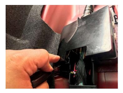
Plug the blue plug of the Double Bypass harness into the WHITE STAR connector that has the green plugs. Plug the black plug into the GREEN STAR connector that has white plugs. Any available slot will work.
