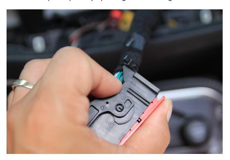
\*\* IF you accidentally placed a wire in the incorrect slot, you will need to remove the red locking mechanism, and gently pry back on the black tab that holds that pin in place, as shown:
