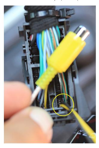
Insert the AUX1 - Front Camera (Red RCA) harness into pins 24(Green) and 25(Black)
