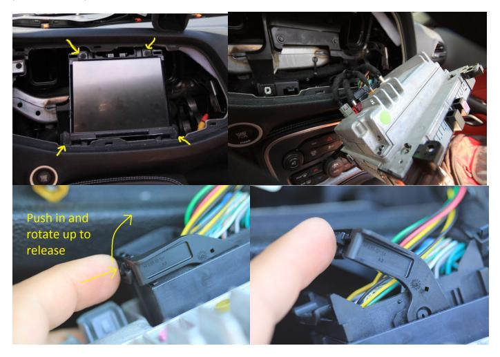
Step 3: Insert harness pins into the radio harness connector. Here you will pry forward the red locking mechanism and place the Z Auto harness pins into their respective cavities. They can only go in one way, and snap into place when inserted. If they won't' fully seat, you may need to use a small screwdriver or tweezers to help push the pin in.
