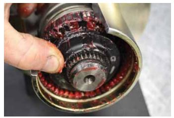
10. While fully compressing the assembly install the axle snap ring if applicable. Assure the snap ring fully seats into the groove on the outer shaft. If no outer snap ring groove exists proceed to the next step in assembly.
