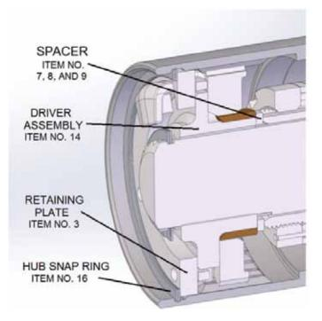
There are three spacers included with the YHC70007 kit which are different thicknesses; small, medium, and large.
