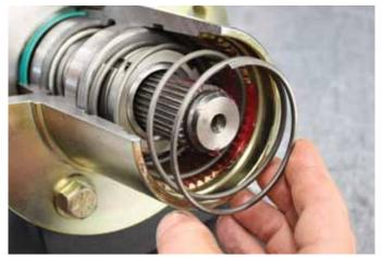
7. Coat the spacer with high pressure grease on all surfaces. Assemble spacer over the outer axle and seat it against the spindle or snap ring. Different spacer heights are available for different hub applications. Verify the Lockout assembly part number and proper application before moving forward.
