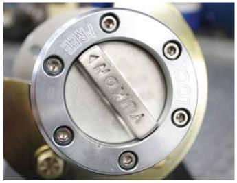
Note: The arrow of the selector must align to the center of the "FREE" and "LOCK" indicators. If the arrow does not align to the center of the indicators, check all installation steps. Extra force may be required to fully turn the selector handle.
