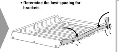
NOTE: Install brackets a minimum of 3 spaces apart and not over a joint.
