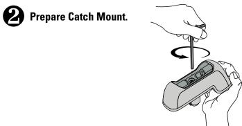
Using the hex wrench fully open both Catch Mounts by turning the screw counter-clockwise. For Outback 2010
