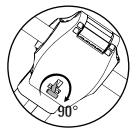
Tighten the knob, but don't tighten all the way. Final tightening will occur after rear clamp has been installed.
