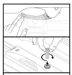
**Note:** If you accidentally remove the clamp nut, compress the clamp and thread the nut back onto the threaded post.
