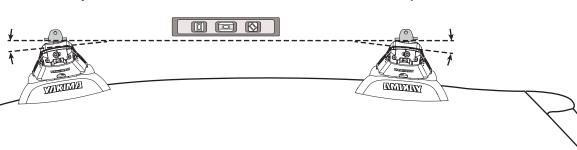
A. Install the bracket from your LockNLoad Platform, the plate, and nut insert as shown. Set the tower pitch. Tighten to 3.5 Nm using the torque wrench.
