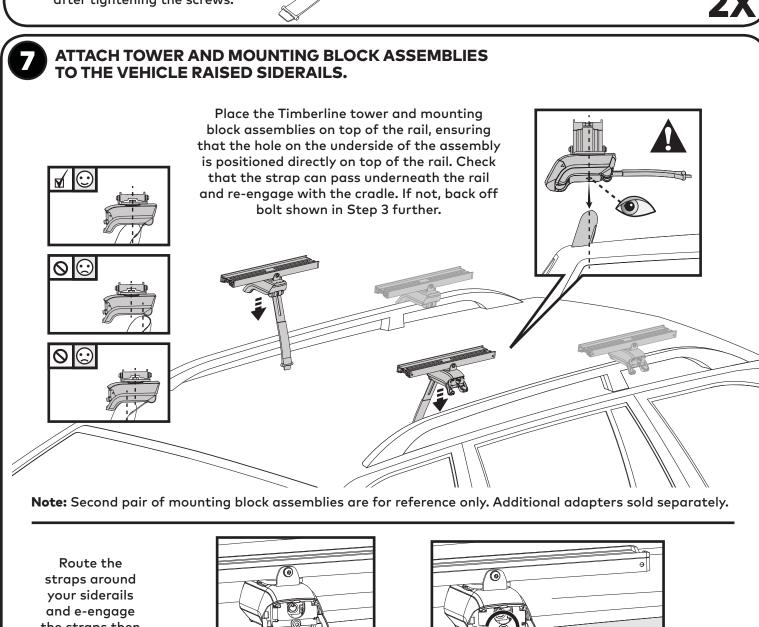
the straps then tighten the bolts until the assemblies are stable on the rails but DO NOT TIGHTEN them completely.
