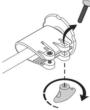
Diagram 2 shows a close-up of the end of the bar. A knob is being turned counter-clockwise, as indicated by a curved arrow. A carriage bolt is being unscrewed from the end of the bar, as indicated by a straight arrow.
