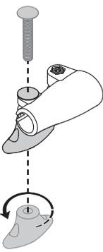
Diagram 4 shows a close-up of the end of the bar. A carriage bolt is being inserted into the hole, and a knob is being turned clockwise, as indicated by a curved arrow.
