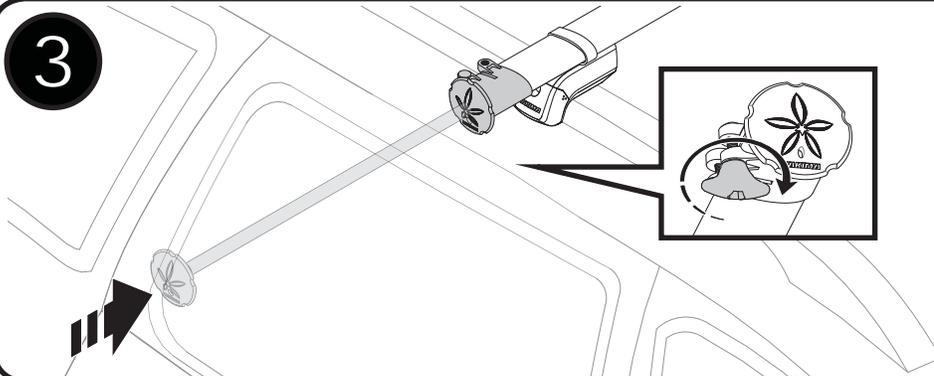
Loosen the knob and push the extension back in. Tighten the knob again.
