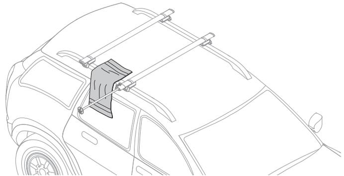
Note: If the clamp becomes disengaged from the end of the crossbar, tighten the clamp bolt as in step 5.
