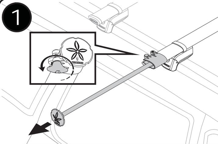
Loosen the knob so the the bar can slide. Extend the bar away from the car. **TIGHTEN THE KNOB.**
