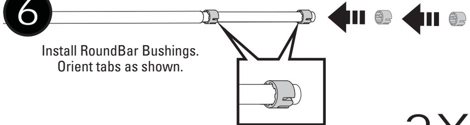
Diagram 6 shows the long metal bar with a knob at one end and a cap at the other. Two small cylindrical bushings are being slid onto the bar, as indicated by arrows. A callout box shows a close-up of the bushing being installed, with an arrow pointing to the tabs on its side.
