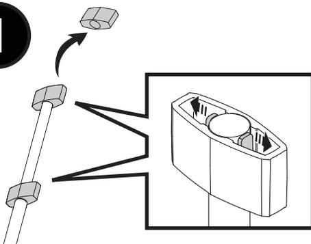
Flex the tabs and remove the rubber inserts.
