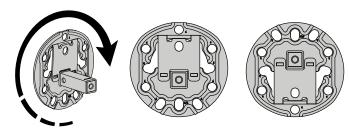
Mounting plate rotates to accommodate different vehicles. Use the numbers on the mounting plate to guide you. 5 =five-hole wheel, 6 =six-hole wheel.
