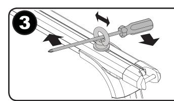
Position the Eye Bolt then tighten it using a screwdriver to gain enough leverage to tighten it to 8-10 Nm (6-7.4 ft-lb).
