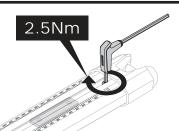
• Reinstall the end caps with the 4 mm hex wrench, and tighten to 2.5 Nm.
