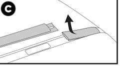
At the ends of the ditch molding, use caution to not disturb any factory applied anchors for the weather-stripping.
