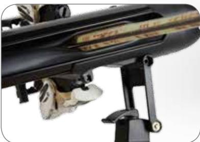
Integrated ski lift allows for rooftop clearance for snowboards or tall bindings.
