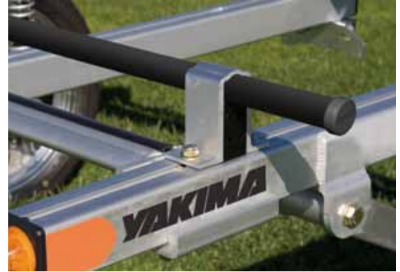
Tighten to 23 ft. lbs (31N-m).
