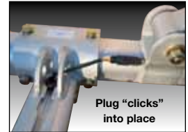
9F Side Rail Connectors Mated
