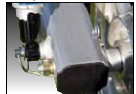
7E Tighten to 57 ft. lbs. (77N-m), right Wheel Block shown
