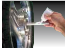
7C Grease Wheel Axle Bolt before and after insertion
