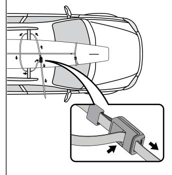
Push and hold button, then thread strap through underside, and out the front of RipCord lock.
