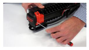
Take product and remove both Xray Vision branded end caps (one on each end of the driving light) using a fine blade screwdriver
