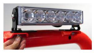
Position driving light in desired mounting location, then loosely fix main mounting bolt washers and nuts to hold the light into position (do not tighten at this stage as mounting bolts need to be left loose until final alignment adjustments have been made at the end of the installation process)
