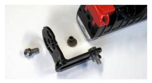
Identify the mounting bracket that contains the adjustment device, remove centre bolt and mounting foot, while taking care not to lose the adjustment cam
