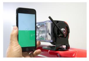
For up/down alignment, use a 6mm Allen key to turn the adjustment cam up or down until you reach the desired beam angle of 0° (90° to the horizontal plane); many modern smartphones have a leveling App built-in
