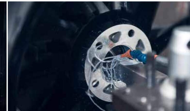
A change in vehicle model usually comes with a change in the center bore of a vehicle's suspension. Custom center-boring produces better ride comfort eliminating vibrations.
