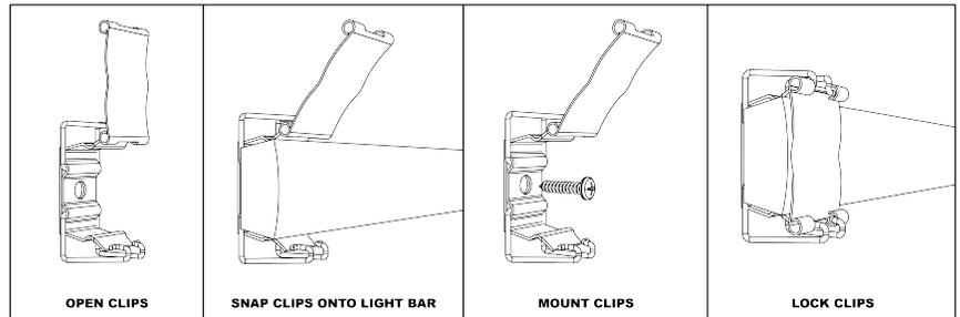
4. **Install light bar:** Snap the light bar into the brackets. With the light bar in place, close the clips and lock into place with the pins. Needle nose pliers will come in handy here! *Please note that the wiring must exit towards the left side of the vehicle.*
