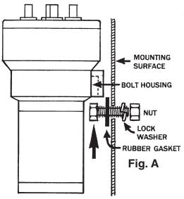
1. Install the compressor in the engine compartment in a dry location and safe from engine exhaust manifold heat. To secure the compressor, drill a 3/16-inch hole through metal and mount compressor vertically (air outlets at the top). Insert head of bolt into the bolt housing and secure to the vehicle referring to Figure A. Use mounting hardward in the order shown – bolt, rubber gasket, mounting surface, lock washer, nut.
