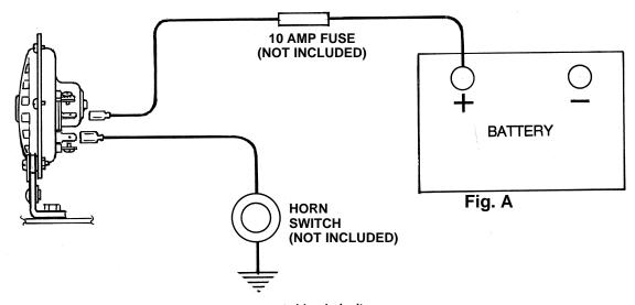
Ground to any metal body bolt that is clean of paint and rust.
