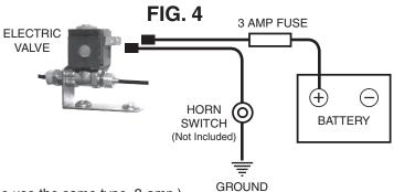
from the power source. (Note: if you need to replace the fuse use the same type, 3-amp.)
