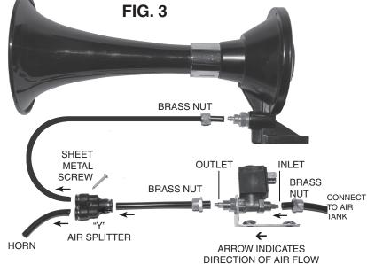
18. The "Y" air splitter can be secured to the vehicle; DIRECT mark hole locations and drill to size: 3/32". Secure air splitter using the sheet metal screw provided.
