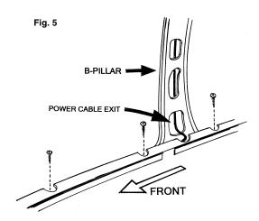
16. Make sure the power cable has been completely pulled into the vehicle, use silicon or similar waterproof material around the grommet and power cable to ensure a waterproof installation.
