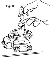
41. Place the lens back on the light bar's base and secure in place using the four screws removed earlier. IMPORTANT: There is a rubber gasket on the edge of the lens, make sure the gasket is positioned properly to prevent water and dirt from entering inside the light. Use care not to over tighten screws that secure lens.
